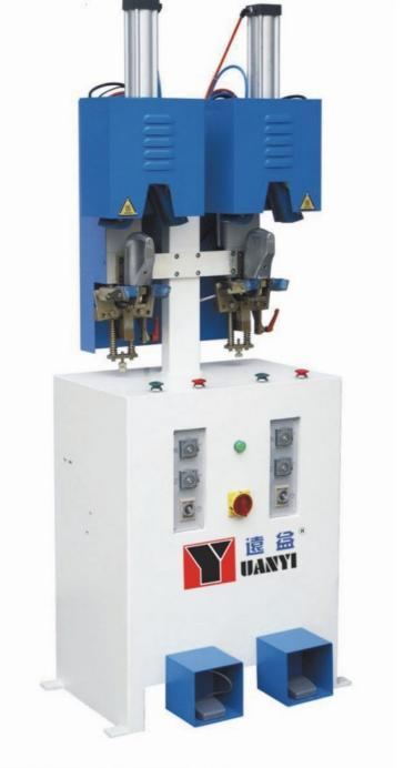
YE-860B 两工位后踵定型机(不摆进式) YE-860B Back Part Moulding Machine (Without Sway Model)
